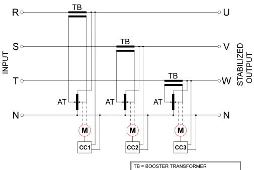
3 PHASE WIRING DIAGRAM EACH PHASE REGULATED INDEPENDENTLY TB = BOOSTER TRANSFORMER
