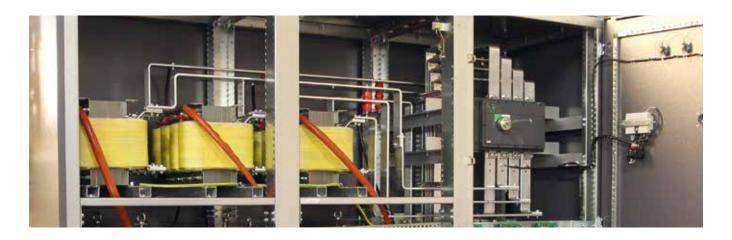
The stabilizers of high-power series, BST-TH, range in power from 400 kVA to 3000 kVA and consist of motorized columnar type variable autotransformers which are contained in a stable built-in case disposed under the base to allow for easy material handling.
