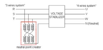
The stabilizer can works even in an unbalanced loads condition.
