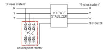
The stabilizer can work even in an unbalanced loading condition provided the power rating of each phase is not exceeded.
