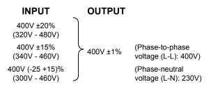
The adjustment of the output accuracy is performed by the electronic card independently on each phase and can be adjusted manually using terminal P1 on Belotti card type BHV.
